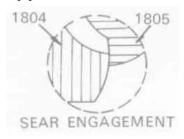
Middle Screw (p/n'1808): Over travel adjustment. Turn the middle screw clockwise to reduce or counter-clockwise to increase over travel of the trigger (p/n#1804) beyond the point where there trigger releases sear (p/n'1805). The middle screw can be turned clockwise too far which will prevent gun from firing. It is recommended that over travel be minimal for best trigger feel. The factory presets the over travel for about 0.25"
